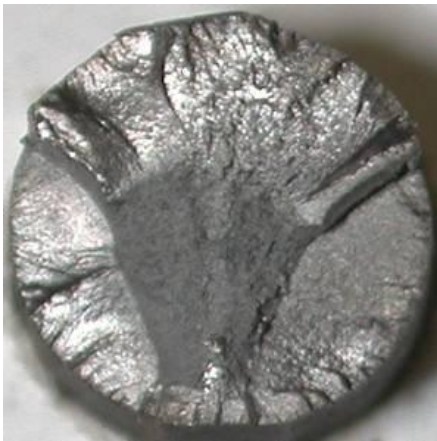
Figure 6. Tip of fractured specimen of medium carbon steel
