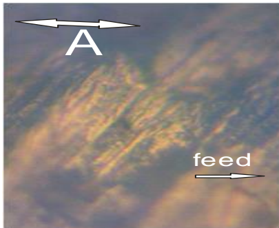
Figure 4. Photomicrograph: specimens of medium carbon steel after machining
