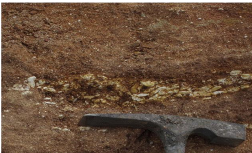
Fig. 4.8. Ferruginized sandstone with a basal gravelly bed at km 5 Leru/Isuochi junction, along PH/Enugu expressway
