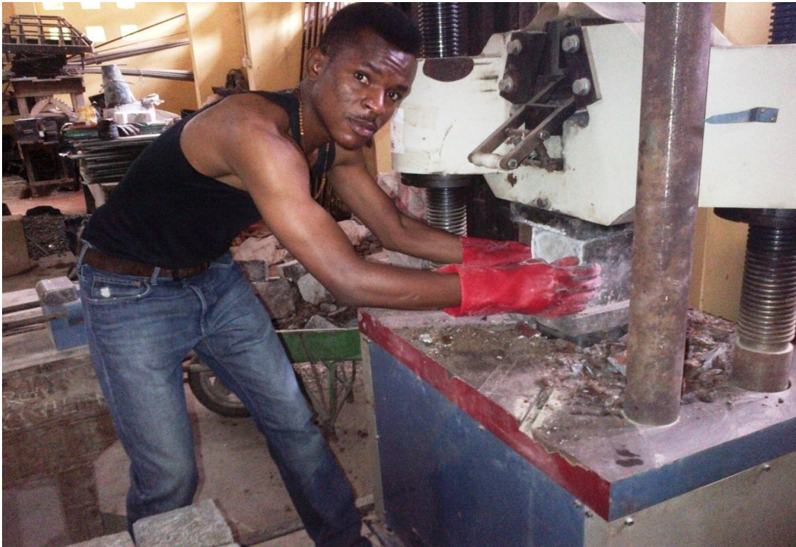
Plate B.13 Concrete Cube Placed on Crushing Machine
