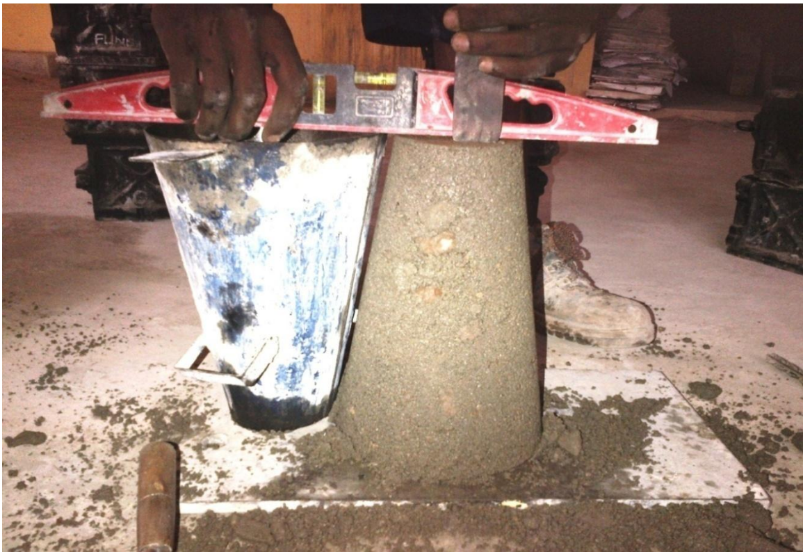
Plate B.10 Slump Test (a)
