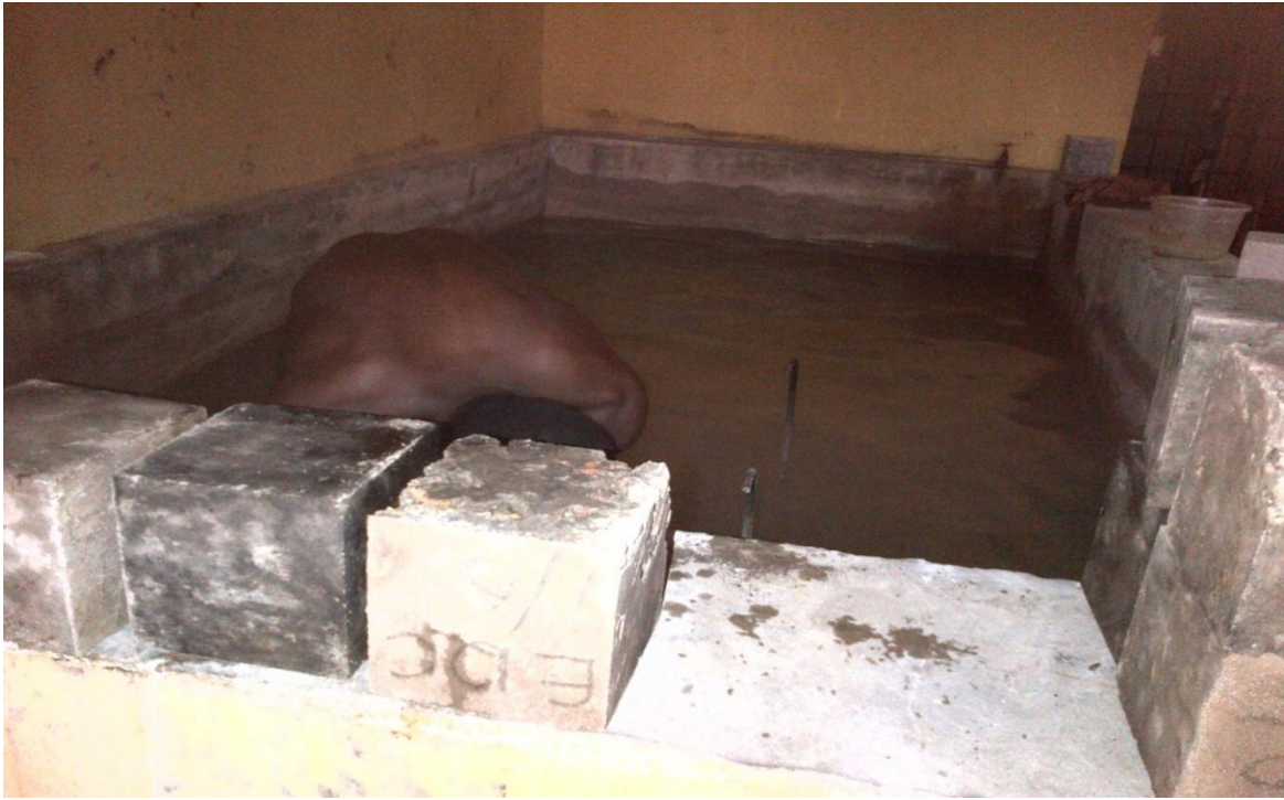
Plate B.9 Cubes Being Immersed in Open Curing Tank
