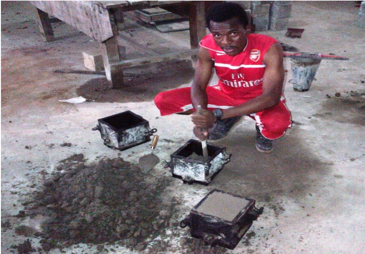
Plate B.7 Casting of Cubes after Mixing
