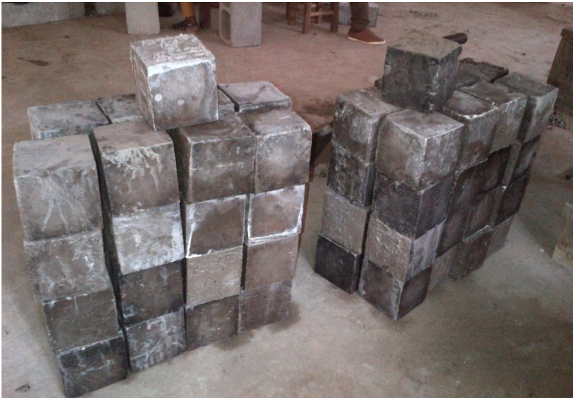
Plate B.12 Cubes Ready to be crushed
