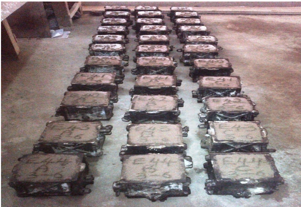
Plate B.7 Casting of Cubes after Mixing
