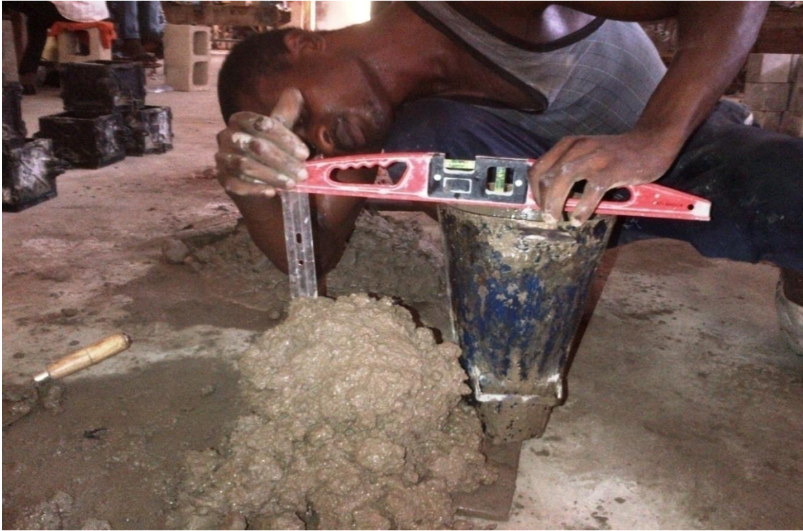
Plate B.11 Slump Test (b)
