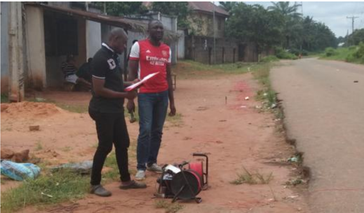
Figure 3.2b: Field Picture of Geophysical Study of the area using direct current resistivity Method.
