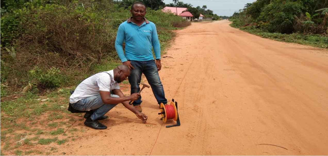
Figure 3.2a: Field Picture of Geophysical Study of the area using direct current resistivity Method.
