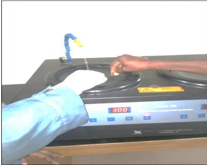
Plate 7.1: Test running the Metallographic Lapping/Polishing machine (UNIPOL 820)
