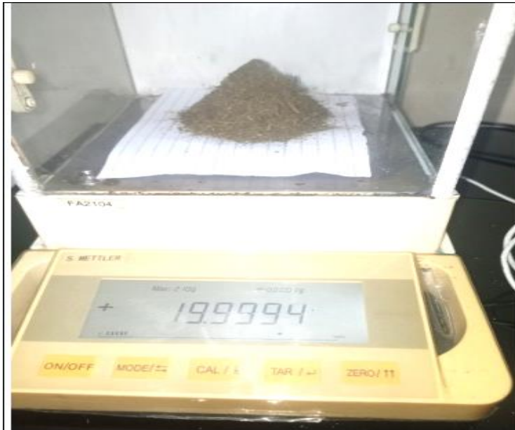
Plate 7.3: Using the FA2104 Electronic weighing balance to measure grinded MPL samples for preparation of extract-based corrosion inhibitor.
