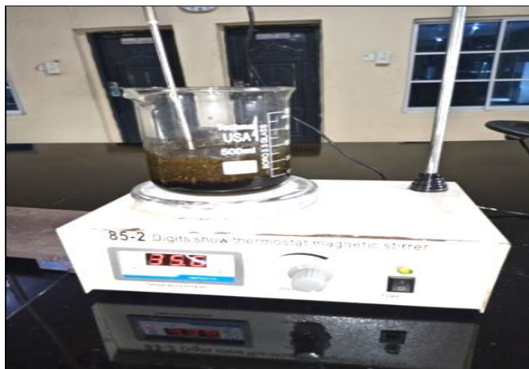
Plate 7.4: Using the magnetic stirrer to stir the the sample of MPL in ethanol to extract the inhibitor
