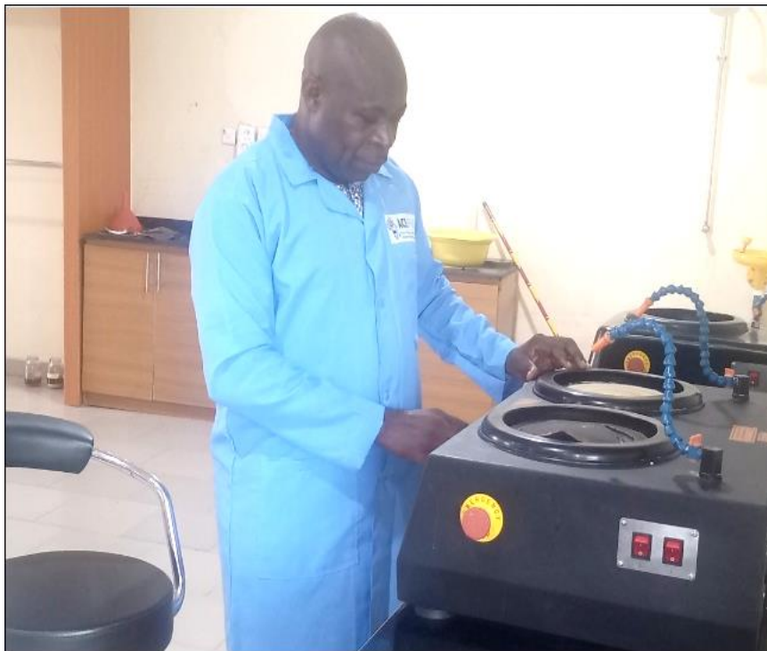
Plate 7.2: Mr. IdemaOsuaniFyneface Using the Metallographic Lapping and Polishing machine(UNIPOL 820)to polish test coupons.
