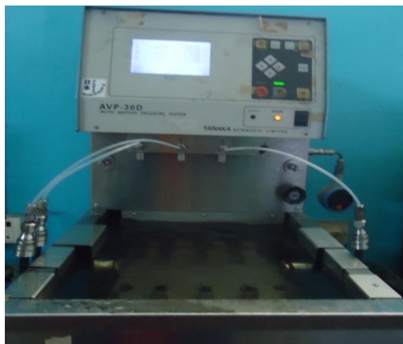
Plate 3.26: Auto Vapor Pressure Tester
