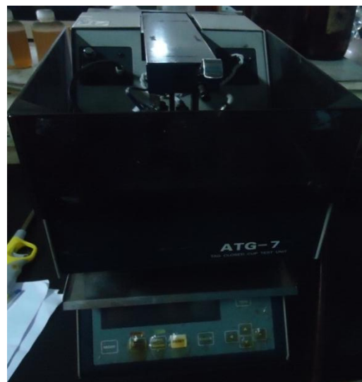
Plate 3.27: Auto Ignition Point Tester
