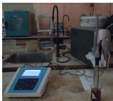
pH Reading (Jenway pH meter Bibby Scientific LTD. UK)
