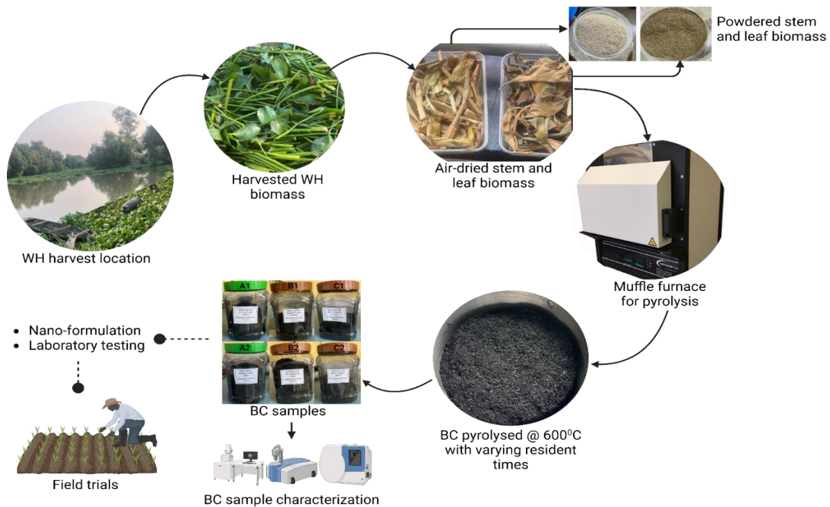
Figure 3.3: Process summary for WH upcycling to produce BC for nano-enabled biofertilizer formulation
