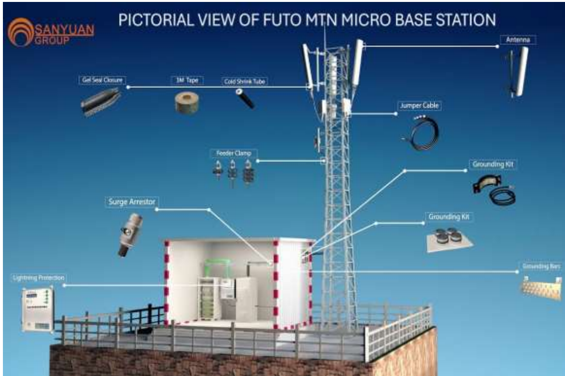
Figure 3.2: pictorial view of components at the sample micro base station. Source: MTN, 2019
