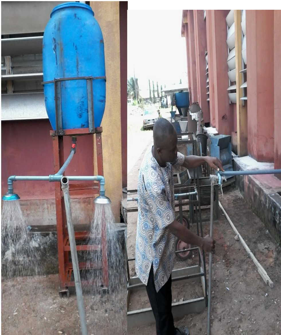
Plate 11: Coupling of the Rainfall simulator
